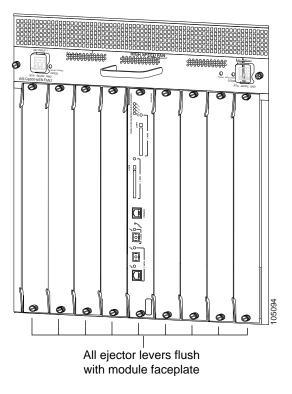
Figure 17 Ejector Lever Closure in the Chassis
